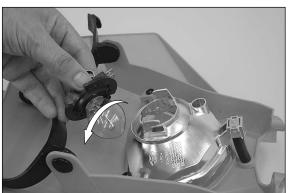
Slightly depress the bulb, turn it approx. 30° counterclockwise and pull it out
